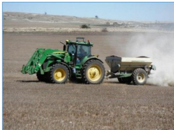
**Figure 3: Applying lime according to pH zones**
