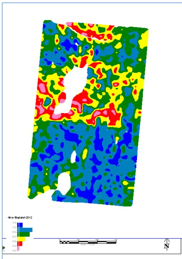
The maps produced by the Veris® machines can be quite detailed (8 -10 points per hectare) and will pick up small areas of low and high pH soils. The map from the soil sampling units (generally less than 2 points per hectare) will be less detailed but will pick up broader soil pH zones.
